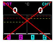
The red cross over the display means the TC-4 has lost communications with the external RDAC unit. Check the wiring between the TC-4 instrument and the RDAC unit. This error message is only available when the external RDAC is selected as the thermocouple data source.
