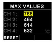
This display can be accessed by rotating the rotary control during the normal display mode. Press the F1/Up button when the max values display is showing to reset the maximum values to the current temperature values.
