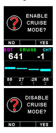
Once in the cruise, press the F2/Down button to enable the Cruise Mode. The "CRUISE" label is displayed at the top of the main display to clearly differentiate it from the normal operating mode. All EGT and CHT readings are immediately sampled as reference temperatures for the cruise.
