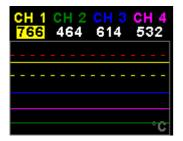
This display can be accessed by rotating the rotary control during the normal display mode. The trend graph displays the last 100 seconds of temperature readings.
